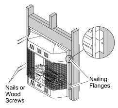
Figure 7 - Attaching Fireplace to Wall Studs
